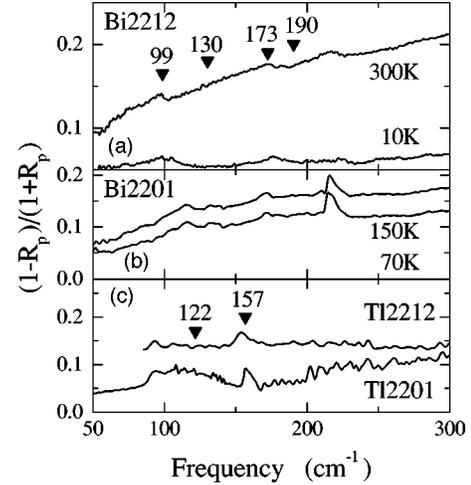
FIG. 5. Function  $(1 - R_p)/(1 + R_p)$  for Bi2212 (a), Bi2201 (b), and Tl2212 and Tl2201 (c) for different temperatures in comparison with the positions of the resonances observed by the intrinsic Josephson junction spectroscopy: (a) for Bi2212 (marked by triangles and the corresponding value) and (c) for Tl2223.
