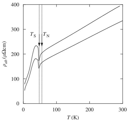
Fig. 1. In-plane resistivities of two representative  $\text{Ca}_3\text{Ru}_2\text{O}_7$  crystals grown by floating-zone method, shown as a function of temperature. Indicated are the observed Néel ( $T_N$ ) and structural transition temperatures ( $T_S$ ).
